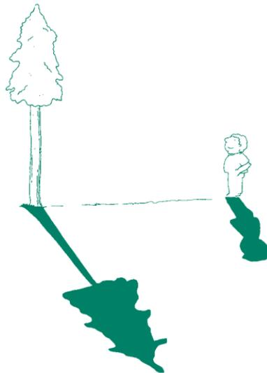
*Incorporating Precision:* You can test the precision of one or all of these methods by measuring a single tree multiple times. For example, use the Shadow & Partner Method at different times of day for a single tree and compare the tree heights you calculate. Think about why you may calculate different heights for the same tree.
