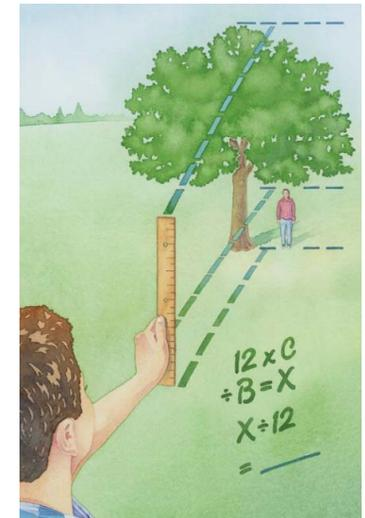
4. Plug your three numbers (A, B, and C) into this equation and calculate the tree's height tree, in inches (H):
